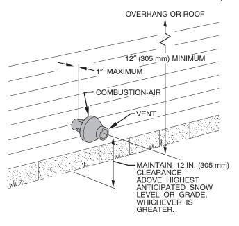
Fig. 41—Concentric Vent and Combustion-Air SideTermination
